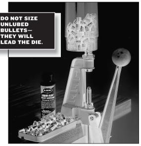
Very large and long bullets with a flat nose may stack and push the cover off the box. A washer under one edge of the press base will tilt the press sufficiently to prevent stacking.
