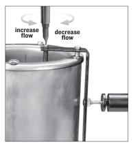
With an ingot mold placed under the pour spout, lift the pour knob and observe the flow. Rotate the valve rod clockwise to decrease flow. As the metal is consumed, you will need to rotate the valve rod counterclockwise to maintain a uniform flow. Do not rotate the valve rod too far counterclockwise as continuous flow will occur. As the valve spout ages, it may corrode or accumulate debris. Should your valve begin to drip,
