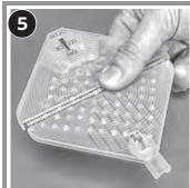
Unfold tray and place on top of box of 100 primers.
