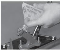
Slide the primer tray into the adapter, slide the flow control to ON, and watch the flow of primers from tray into adapter. Primers may bridge, tap the upper corner of tray occasionally to resume flow.
