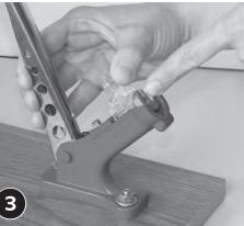
While lifting the lever, slide adapter into the body of the tool far enough to install priming tool shell holder.
