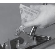
Lift the lever against the stop to feed the staged primer to the primer pin. Place a de-primed case into shell holder. Depress lever with index finger to seat primer. Primers should be seated flush to slightly below flush of the case head. Lever will not bottom out and you will quickly learn to feel when primer has reached home by the increase in pressure on lever. Be sure to lift lever against rubber up-stop on every cycle.
