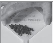
table, shake tray side to side to upright all the primers. Allow cover to naturally fold up, notice how the primers glide across hinge, upright themselves and work their way towards the outlet. Fold and close cover.
