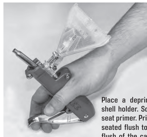
Place a deprimed case into shell holder. Squeeze lever to seat primer. Primers should be seated flush to slightly below flush of the case head. Lever will not bottom out and you will quickly learn to feel when primer has reached home by the increase in pressure on lever. WARNING If you feel an increase in pressure on the lever earlier than normal, you have a problem and continued pressure may result in a primer detonation. Stop pressing and determine what is causing the early increase in pressure. It is likely a tipped primer, a military case that does not have its crimp completely removed, or attempting to prime an already primed case.
