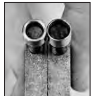
To determine small vs. large lever assembly, note difference, SMALL (left) LARGE (RIGHT)
