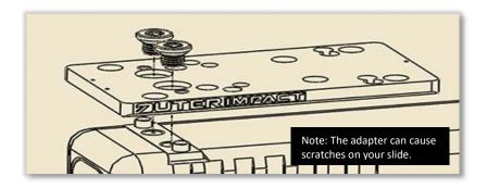
Step 5: Using the screws/pins and the mounting pattern identified, mount the Red Dot sight adapter and torque to 12 in/lbs
